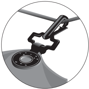
Fastening a net with a bridge clip and a fast connection clasp
