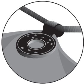
Fastening a net with a bridge clip
